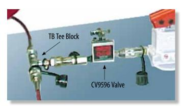
A 100H2 Pump with TB Tee Block, two hoses and CV9596 Load Lowering Valve are recommended for operating two HS10Ks simultaneously.
