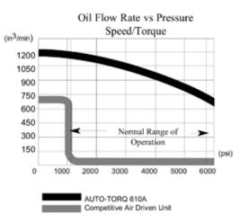
The AutoTORQ power units maintain higher speeds all across the torque range. The competitive pump delivers high speed at 10% of torque then drops to onetenth of the AutoTORQ speed and stays there across the torque range.
