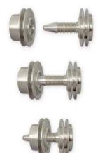
The photos below illustrate the special thread design of the fastener components. To prevent loosening due to vibration or rotation, radial grooves cut in the male components replace the helical threads normally used in fasteners.
