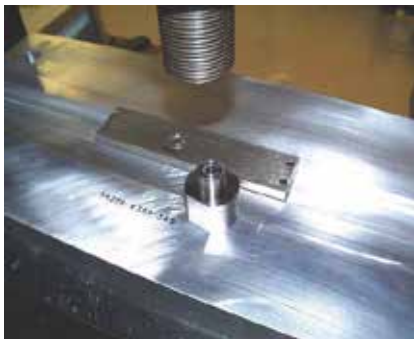
Figure 3. Galled Test Button and Block
