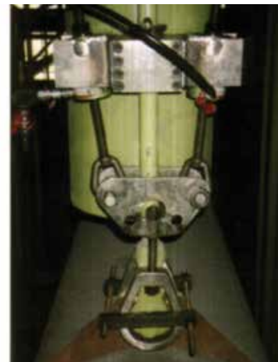
Figure 4. An example of In-Situ Hanger Test Assembly.
