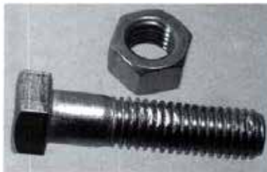
Stainless steel bolt with intentionally damaged threads.
