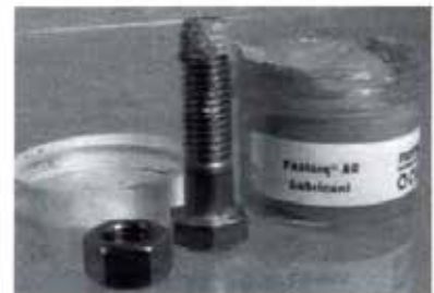
Anti-galling compound placed on bolt's end threads.
