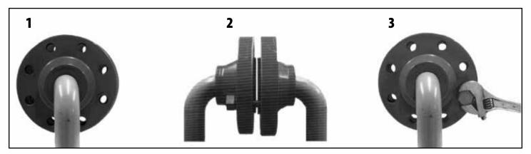
Simply find a bolt hole that is aligned enough for the tapere d shaft to fit through and turn.
