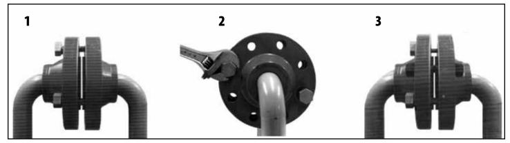
If necessary, use a second tool and turn until the bolt holes are in alignment, then insert flange bolts.
