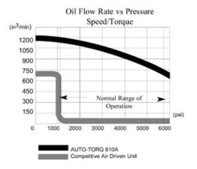
The AutoTORQ power units maintain higher speeds all across the torque range. The competitive pump delivers high speed at 10% of torque then drops to one-tenth of the AutoTORQ speed and stays there across the torque range.
