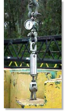
With ZipCONNECTOR, a standard threaded lifting eye can be used to retrieve or abandon objects of various sizes & weights.
