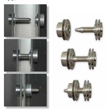
The photos below illustrate the special thread design of the fastener components. To prevent loosening due to vibration or rotation, radial grooves cut in the male components replace the helical threads normally used in fasteners.
