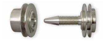
As you can see in the photo below, the female segmented threads are held together by the garter spring. The garter spring keeps the concentric threaded female segments around the male component. Once inserted, any force pulling the make component will cause the female to clamp tighter due to the chamfered angle cut in the leading end of the male threaded segments and the corresponding cut in the ZipNut body.
