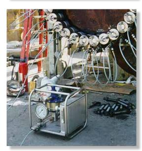
Fastorq Model HTP-2000 is powering 28 ZipTENSIONER Stud Tensioners, size 2 1/2".
